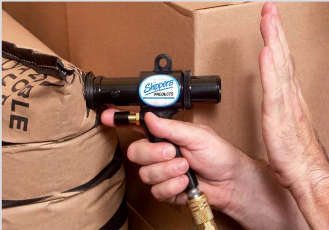
Traditional inflators do not prevent over-inflation and run the risk of bag bursting during inflation. When used properly, the Super Flow™ prevents over-inflation and fills airbags to optimal pressure ensuring ideal load securement.
